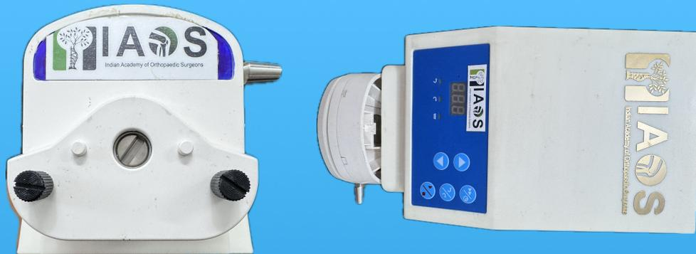
Special IAOS EBOO perfusion machine capable of 0 to 80 ml per minute of blood perfusion, with precise 0.5 mm controls.
